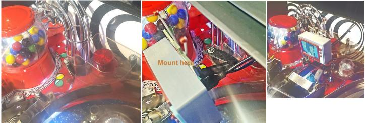
If you wish to mount the video player in a different location or different pinball machine, you can make a custom mount using the 0.8 to 1mm steel wire.
